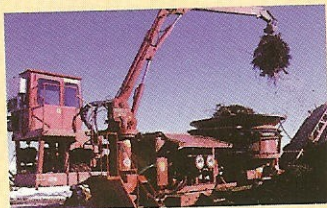
A mobile grinder is brought to the dropoff site to process slash.
